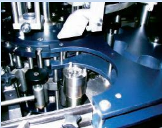
Bottle capping machine, resists effects of foam cleaner
