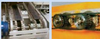
Locking assemblies connecting sprockets to conveyor shafts
