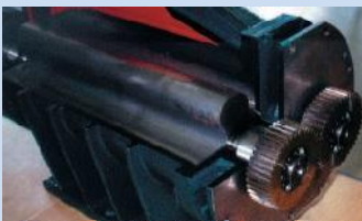
Locking assemblies on the drive side of a compressor
